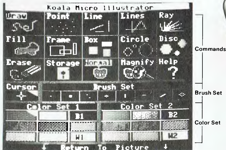
Above: The Koalapad's drawing facilities, as displayed on the screen. Right: The Koalapad.
